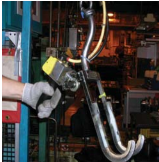
Certified Magnetic Particle Test and Liquid Penetrant Test offered to detect cracks and discontinuities before they become a problem.
